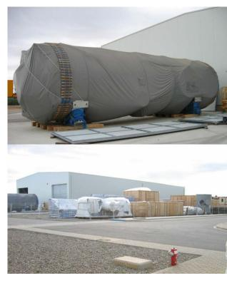
The equipment is stored in an ad hoc warehouse complying with the manufacturer's storage and maintenance conditions
